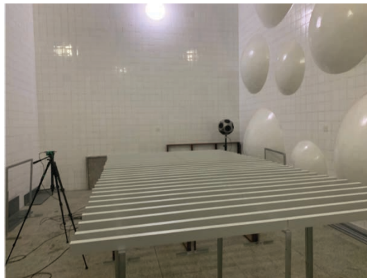
Figure 4. Reverberation room method for sound absorption coefficient testing
